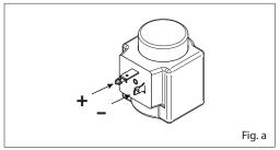
When - (minus) is supplied to the right terminal pin and + (plus) to the left (see fig. a), the valve plate is pressed down against the pilot orifice (4) by the armature spring (2).
