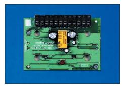
The SNM800 is a remote addressable sounder circuit output device capable of switching sounder and speaker circuits up to 2A @ 24V d.c. or provide a monitored output facility for other applications. These can be used in addition to the two sounder circuits provided as standard on most MX detection panels.
