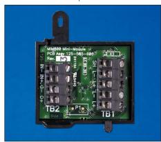
The MIM800 is a small MX addressable module designed for monitoring a single input circuit. The MIM800 can monitor normally open or normally closed inputs and provides open and short circuit monitoring of the line.
