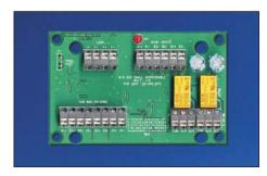
The MIO800 is a general purpose interface module for use with MX Technology<sup>™</sup> fire detection systems. It allows multiple input and output connections to be made between external equipment and the MX Digital loop. Three inputs and four outputs are provided. Each input and output can be programmed independently using the MX Consys configuration tool to provide customised functionality.
