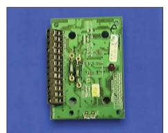
The DIM800 is designed to power and monitor a circuit of low voltage conventional detectors and callpoints. The detection circuit is powered from an external 24V d.c. supply and is reset by the MX addressable panel. The DIM800 monitors the external 24V d.c. and provides a fault signal if it is lost. The input detection circuit can be wired as one or two spur circuits (Class B), one loop configured circuit (Class A) or one 4 wire detection circuit.
